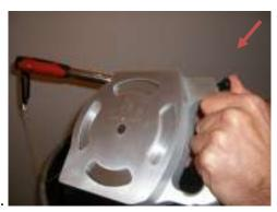
Press & hold the cable reel locking thumb button at top of handle.
