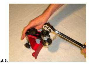
Once removed from base, turn ratchet wrench sideways and slide from spring cradle.
