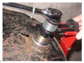
Place tool on drum ensuring it aligns with the bung cap.
