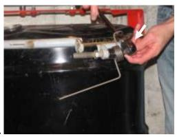
Press and hold release button on back of ratchet head while pulling ratchet from socket.
