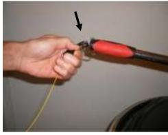
Clip J & D cable reel onto the end of handle and unroll the cable until the device can be operated from a sheltered location or at a distance which the operator has determined to be beyond the range of the hazards presented by the contents of the drum and the extent of pressurization in the drum.
