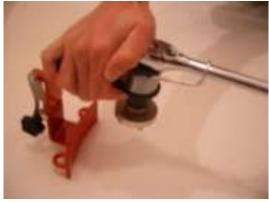
Align ratchet drive with female insert on assembly, and raise ratchet handle until the ratchet drive is firmly seated into the assembly.
