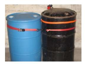
9. Using the two hooks, attach the metal handled barrel stabilizer strap around the upper portion of the pressurized drum and another full, non-hazardous drum or a stationary object such as, a post. Pull excess strap through spool. Pump ratchet handle until strap is taut; do not over tighten. Close ratchet handle to lock in place.
