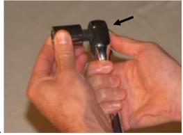
Push button on back of ratchet while inserting magnetic socket. Release button and snap into place.
