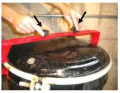
Place the first retainer across the top of drum insuring not to obstruct the retaining ring bolt. Slide the sides firmly against drum and tighten knobs.
