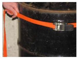
Using the six foot, rubber handled, ratcheting tie down strap, attach hook on ratchet side to the eyelet on base of tool and wrap strap around drum.
