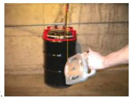
Pull slowly to insure the drum is not pulled over; while pulling listen for the sound of escaping pressure; once the pressure release begins, stop pulling until the pressure release stops and again pull until all pressure release occurs then stop; continue venting the drum in this manner until the retaining ring bolt is completely removed, and all pressure has been released.
