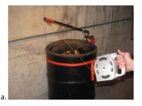
Press & hold the cable reel locking thumb button at top of handle. Pull slowly to insure the drum is not pulled over; while pulling listen for the sound of escaping pressure; once the pressure release begins, stop pulling until the pressure release stops and again pull until all pressure release occurs then stop; continue venting the drum in this manner until the bung cap is removed and all pressure has been released.
