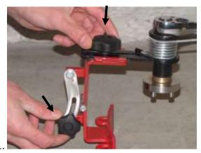
Loosen the two knobs that adjust the tool vertically and horizontally.
