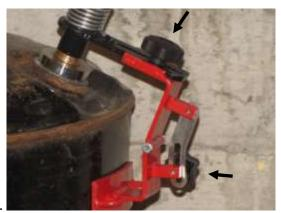
Hold wrench firmly in place while tightening adjustment knobs.
