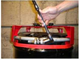
With one hand on the ratchet head, and one hand on the ratchet handle, firmly pull the handle to the left at a 45° angle removing the magnetic socket from the bolt.
