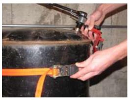
Secure second hook to opposing eyelet. Pump ratchet handle until tool is snuggly secured to drum. Close ratchet handle to lock in place.
