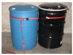
Using the two hooks, attach the metal handled barrel stabilizer strap around the upper portion of the pressurized drum and another full, non-hazardous drum or a stationary object such as, a post. Pull excess strap through spool. Pump ratchet handle until strap is taut; do not over tighten. Close ratchet handle to lock in place.
