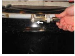
Insert retaining ring bolt into eyelet on ring and turn socket a few times to reconnect the ring.
