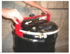
Loosen knobs on the J & D Rigid Retainer. Pulling each side, slide open Rigid Retainer to fit on the drum.
