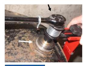
Re-check that the bung driver is firmly seated into the bung cap with the handle to the left side of the operator and the ratchet lever is toward the letter (L) for loosen.
