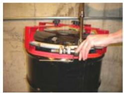
Carefully insert magnetic socket ratchet wrench onto head of retaining ring bolt.
