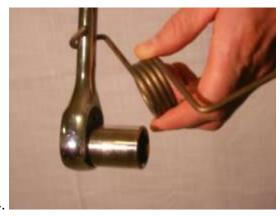
Hook the return lever spring cradle onto the outside of the ratchet wrench handle.
