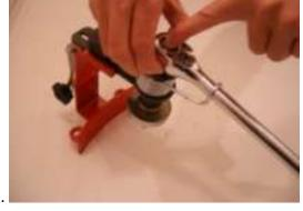
Compress release button, while gently prying fingers between ratchet head and bung wrench assembly base. If ratchet head doesn't come out, wiggle the end of handle while prying with fingers.
