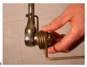
Move the spring cradle down the handle and slide onto socket.
